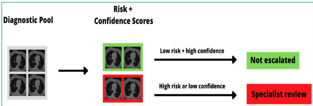
Fig. 3 A sample triage pathway for diagnostics. Each examination is given a risk category and confidence estimate by the AI model, and scans that are deemed high risk or have low diagnostic confidence are
