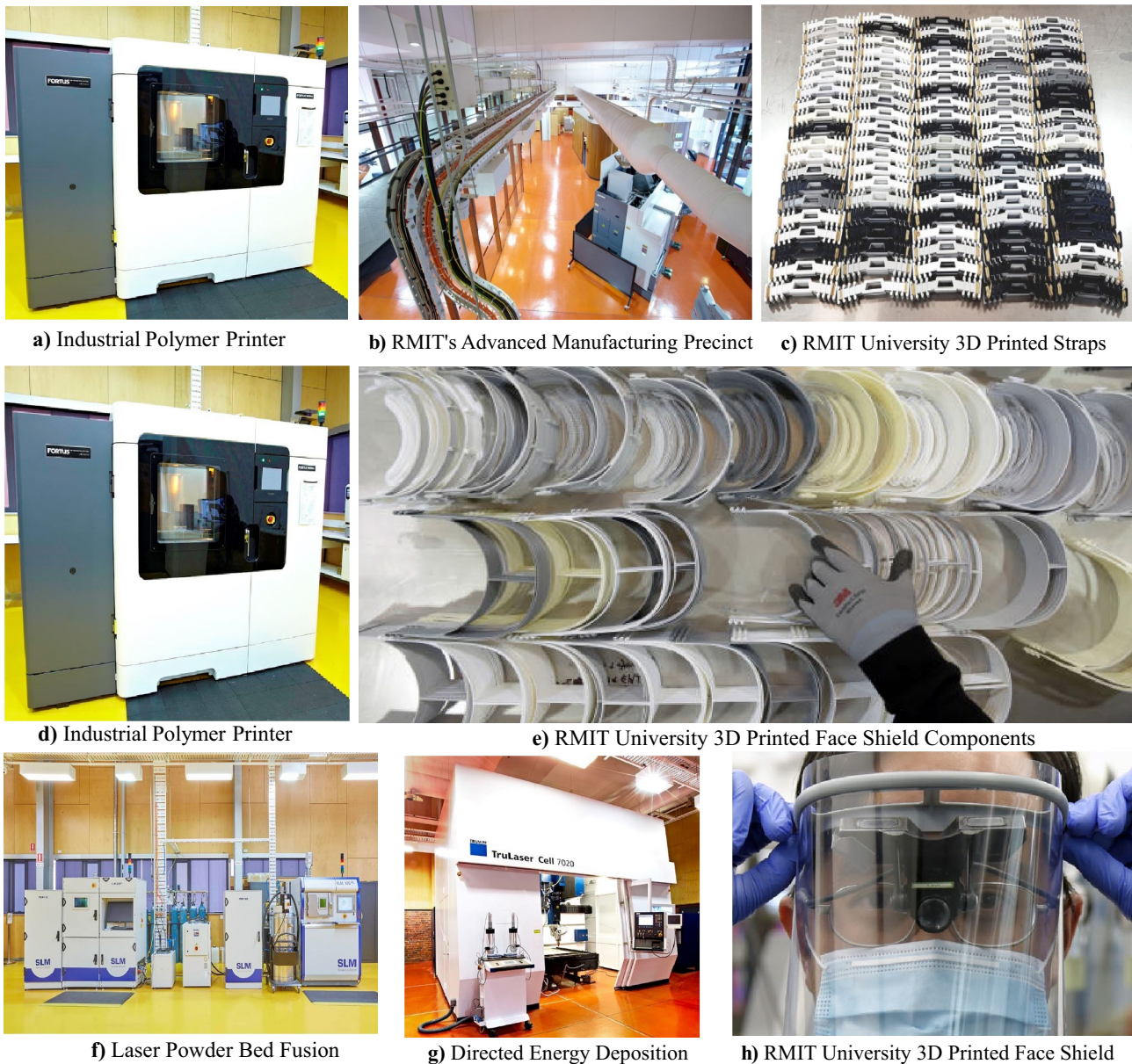
Fig. 5 Face shield and straps manufactured by 3-D Printing at RMIT University in the beginning of COVID-19 pandemic, adapted from [23]
