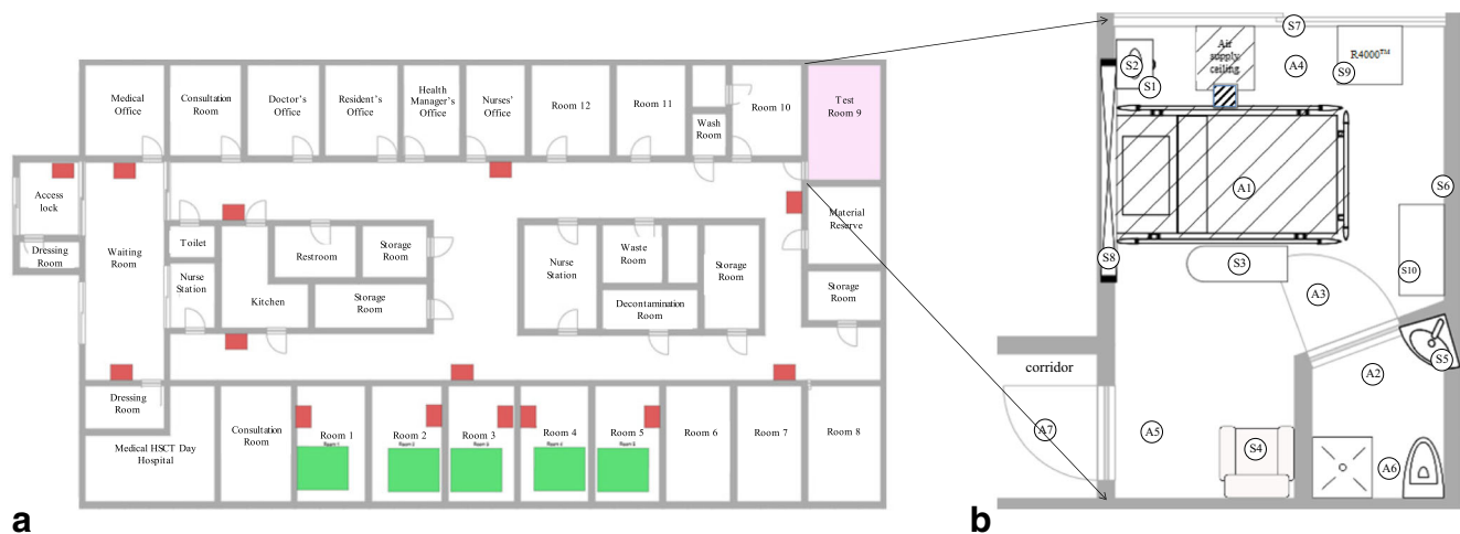
Fig. 1 Map of the adult hematology unit ( a ) and of the test room ( b ). Small red rectangles stand for Plasmair® units. Green rectangles stand for Immunair® units. The hatched area shown in Fig. b is for the air supply ceiling over the bed. The airborne particulate and microbiological
