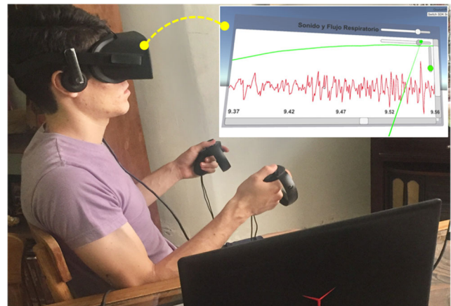
Fig. 4 Illustration of the interactive manipulation of the signals using the VR app and Oculus Rift system
