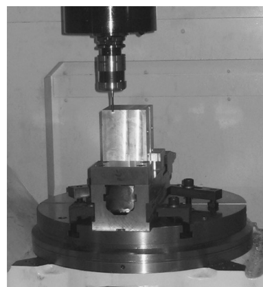
Fig. 4 Square workpiece for calibrating geometric errors of rotary axes [90]
