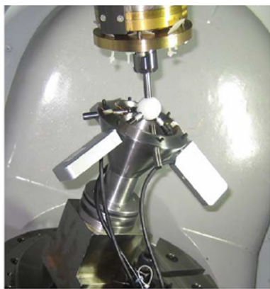
Fig. 8 The prototype setup of the R-test [133]
