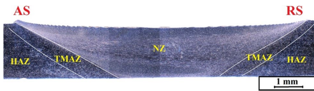
Fig. 6 Cross-section morphology of FSW joint
