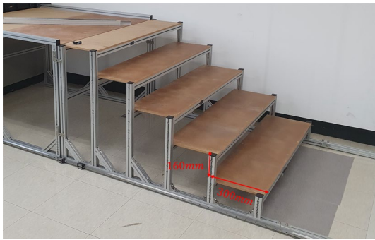
Fig. 8 Test bench (300 mm×160 mm)
