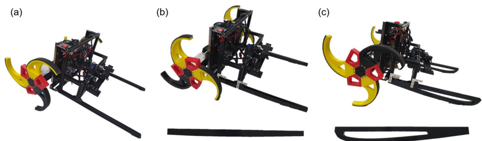
Fig. 7 Prototype robot and blades a LEVO prototype robot b LEVO with B-spline(one control point) blade and its blade c LEVO with B-spline(two control point) blade and its blade
