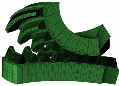
Fig. 10 the FEA model of the SBG transmissions
