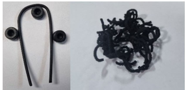
Fig. 5 Four times dispersion of TPU/CNT filament with high CNT wt%: 23.3% (left), 25% (right)
