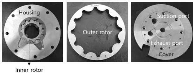
Fig. 23 Prototype of the oil pump with the optimal gerotor with the 2-Ex_Lemniscates
