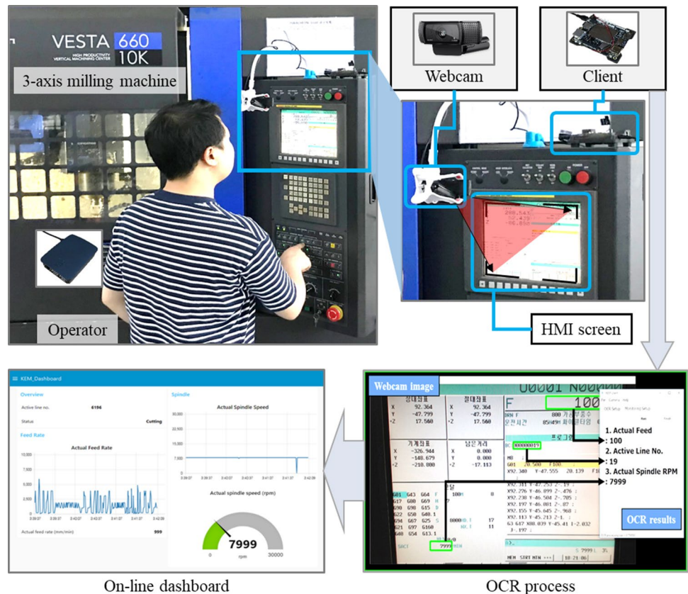
Fig. 7 Appropriate vision monitoring system for old machine tools
