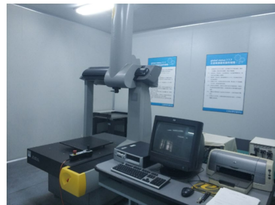
Fig. 3 Global status three-coordinate measuring machine
