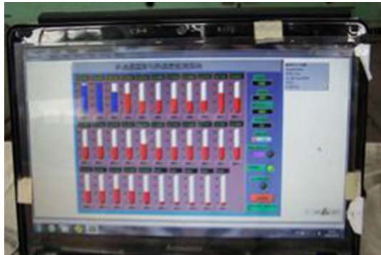
Fig. 19 Multi-channel temperature detection system
