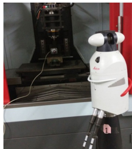
Fig. 9 Geometric error detection of the NC milling machine
