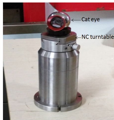
Fig. 4 The precision NC turntable
