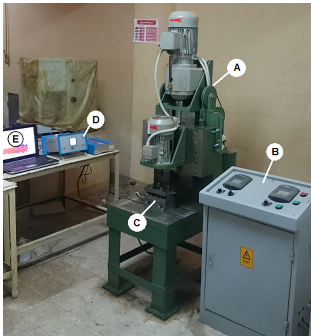
Fig. 2 The manufactured friction drilling machine (a), machine control unit (b), Multi-component dynamometer (c), dynamometer data acquisition and amplifier (d), and laptop (e)
