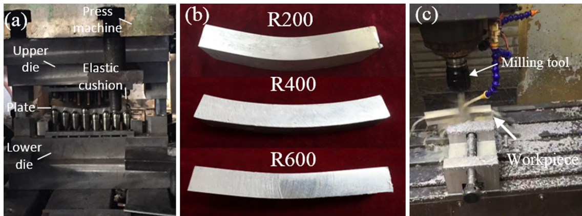
Fig. 4 Milling experiment. a Bending process, b bent plate and c milling process
