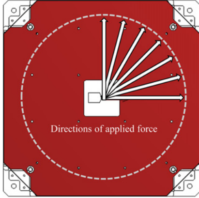
Fig. 6 Applied forces and their directions for stiffness analysis in FEA software (red colored part is moving part which is end-effector)
