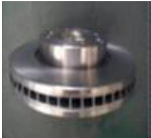
Fig. 15 Newly manufactured brake disc with optimal undercut around the hub
