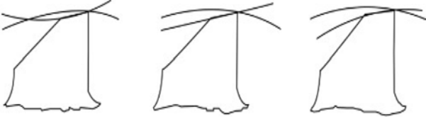
Fig. 9 three types of cutting edges: concave, flat and eccentric
