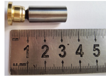
Fig. 10 Photograph of one individual piston-slipper assembly of the investigated EHA pump prototype
