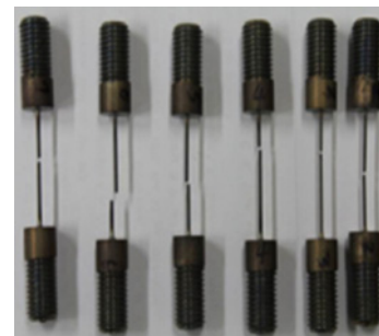
Fig. 7 Specimens after tensile test at 1000 K
