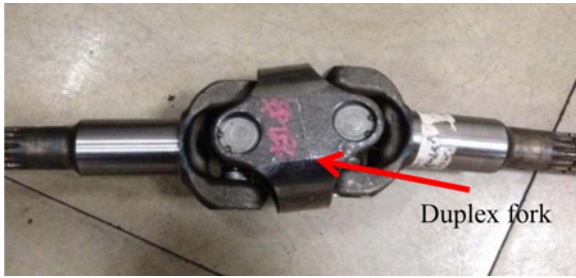
Fig. 1 Typical universal joint
