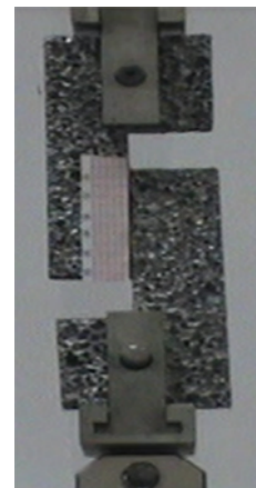
Fig. 6 Test of adhesive strength at bonded interface
