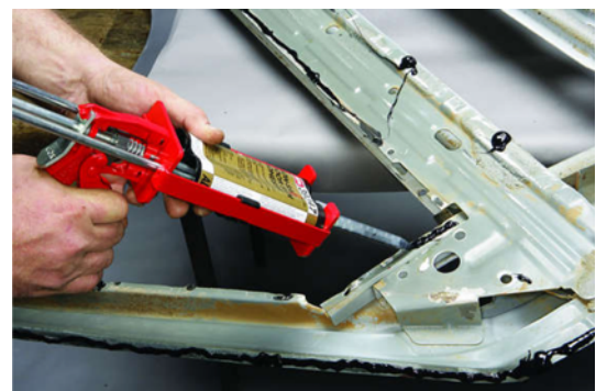
Fig. 3 Application of adhesive structure
