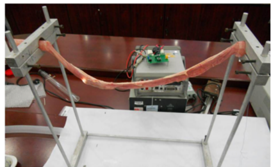
Fig. 18 Locomotion test in excised intestine
