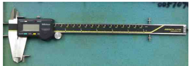
Fig. 7 Mitutoyo digital slide caliper for length measurement
