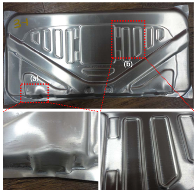
Fig. 12 Partition panel tryout results at tryout condition (c) [(a) Necking, (b) Scratch]
