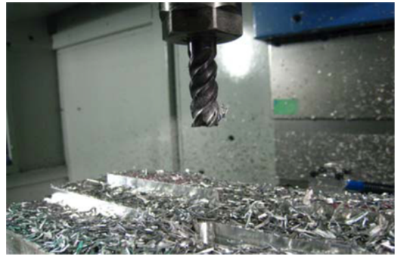
Fig. 13 The cutter with BUE
