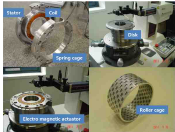
Fig. 5 Photograph of the manufactured components of the variable preload device
