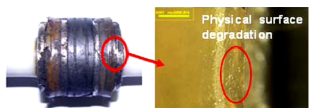
Fig. 2 Seal surface in a failed cylinder
