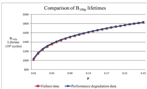
Fig. 6 Comparison of B_{100p} lifetimes estimated from both data types
