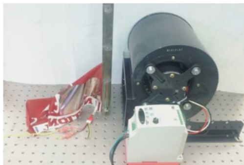
Fig. 7 Bench top wind tunnel setup
