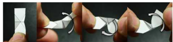
Fig. 7 Spherical six-bar joint based on two-dimensional structure. The structure has three degrees of freedom 17
