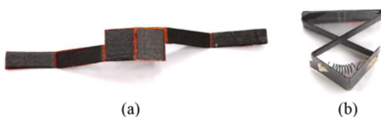
Fig. 14 Fabrication result for the steering jack. Carbon fiber reinforced plastic was used for the rigid component and kapton film for the flexible component
