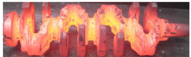
Fig. 3 Workpiece after last forging step
