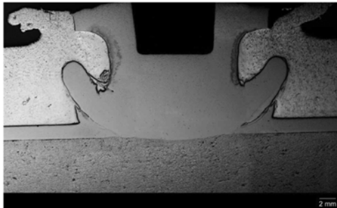
Fig. 6 Cross section of joint composed of A356 aluminum (top), grey cast iron (bottom), and a D2 steel joining bit (center). The intermediate layer of interstitial free steel can also be seen between the aluminum and the cast iron
