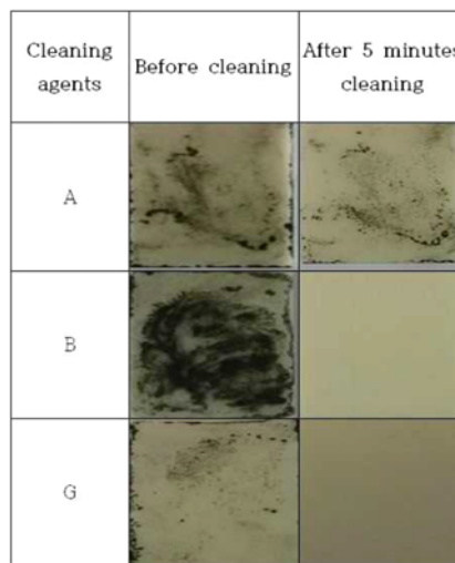
Fig. 4 Comparison of cleaning performance of agents A, B, and G
