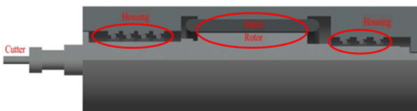
Fig. 7 Heat sources of a spindle-bearing system
