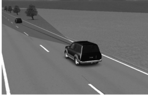
Fig. 14 ACC simulation with CARSIM
