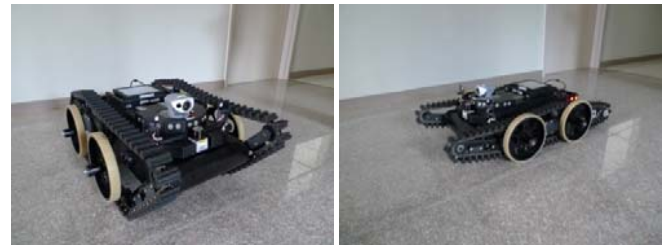
(a) Track driving mode (b) Wheel driving mode
