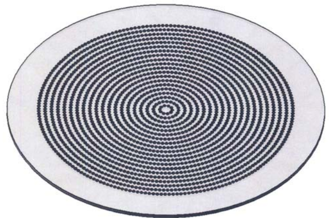
Fig. 5 (a) Apart from Screen Shot 3-D Simulation on Sinumeric 840-D that used the cycle (890) for machining the holes lying in multiple circular arrays patterns (b) Photograph for actual parts used the cycle (890) in machining the holes lying in a multiple circular patterns on Numeripath 800B Giddings & Lewis Machining Center
