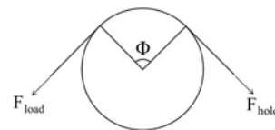
Fig. 2 Forces of the cable on the capstan with a contact angle of pi. In this figure, F_{hold} is amplified to resist F_{load}
