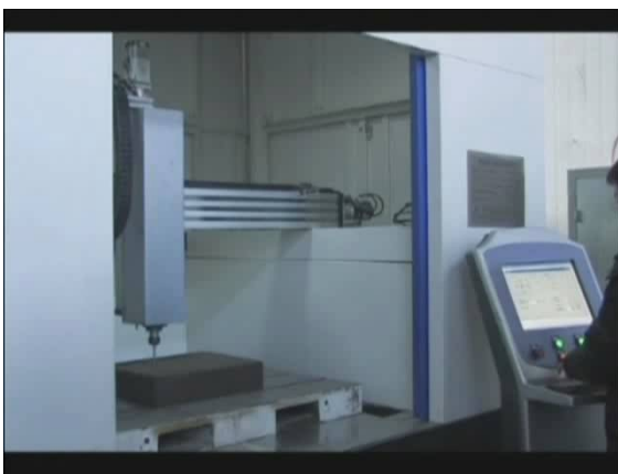
Fig. 5 Digital precision forming machine without pattern casting
