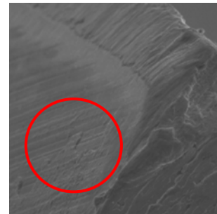
Fig. 7 Coating delamination on flank surface
