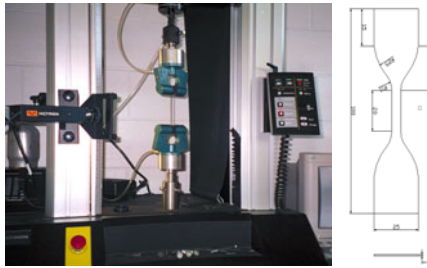
Fig. 1 Uniaxial tension test equipment and specimen
