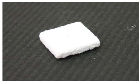
Fig. 5 A multi-layer specimen produced by bioceramic
