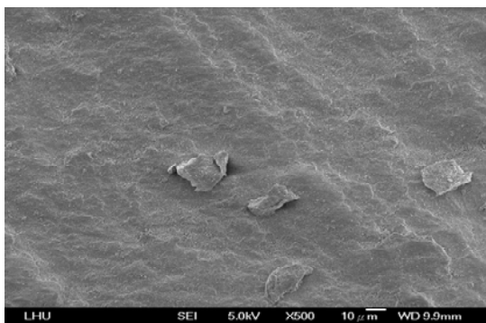
Fig. 3 SEM image showing fracture surface morphologies of the bioactive-ceramic specimen
