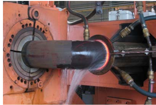
Fig. 21 Apparatus for high frequency induction heating and dynamic reverse moment
