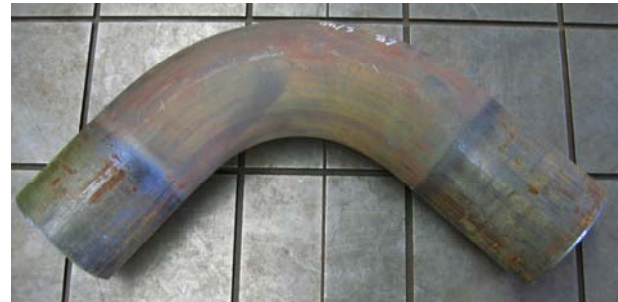
Fig. 22 Photograph of the pipe-bending product
