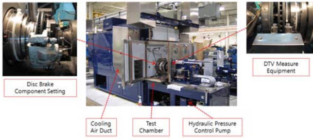
Fig. 2 Configuration of automotive inertia brake dynamometer model 300
