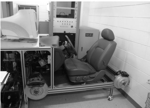
Fig. 5 HILS system for the simulation test
