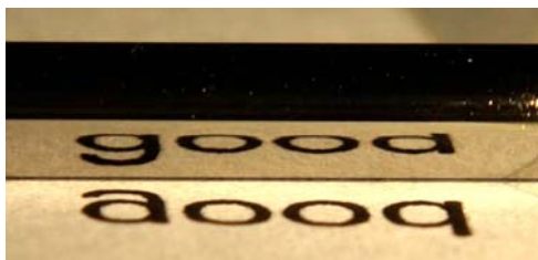
(b) After micro machining (20,000 rpm, 10 Hz, 0.5 \mu\text{m} )
