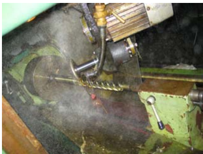
(b) Grinding machining of the female rotors
