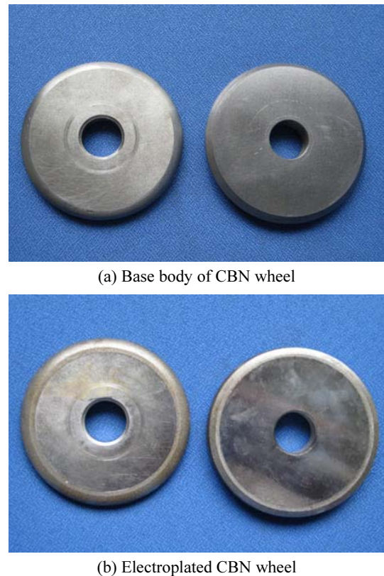
Fig. 6 CBN wheel for machining the rotors
