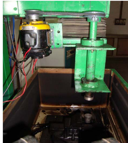
Fig. 4 EDDFG set up assembled on EDM machine
